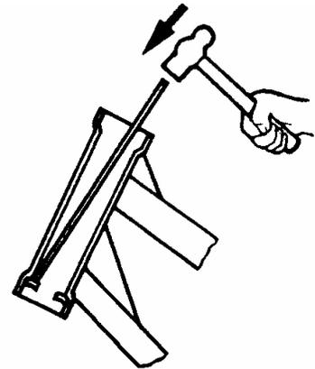
*Tip: before removing the fork legs from the stock trees make sure you break loose the original fork tube caps, but do not remove them from the tubes.*
